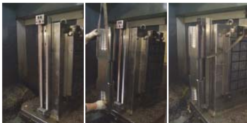
Example of piece differently fixed which closing system results simple despite the piece measures 700mm. JVONNE vises measure till 900mm with 800mm of grip.
