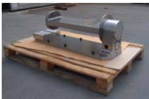
Column-frame for 4th axis divider with counterbearing equipped by pneumatic disk brake.
