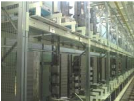
36 pallet plant completely equipped with JVONNE multi-grip cubes octagonal and triangular. Grip capacity until 2 pieces dim. 160x160x500 in first and second phase in one unique 500 cube pallet.
